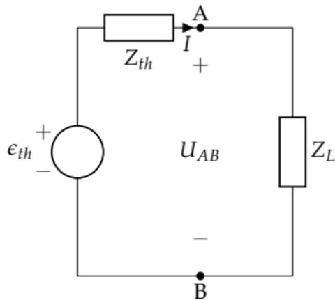
$$P_L = \frac{\epsilon_{th}^2}{|\bar{Z}_{th} + \bar{Z}_L|^2} \cdot R_L \left. \vphantom{P_L} \right\} \bar{Z}_L = \bar{Z}_{th}^* \rightarrow \boxed{P_L = \frac{\epsilon_{th}^2}{4R_{th}}}$$
